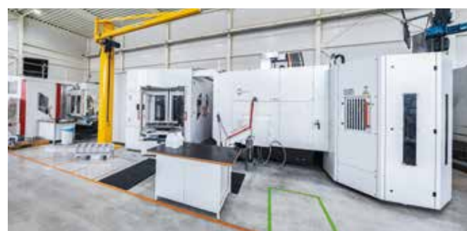
top The nine-metre-high ceilings of the workshop almost make the C 650 U with HS flex heavy automation look small; the robot-automated C 30 U is visible in the background.
