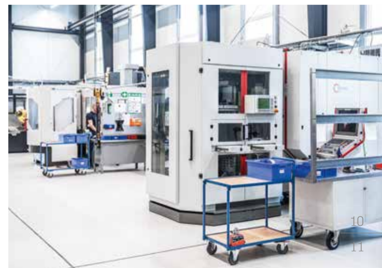
top The handling system at the C 22 U (at the front) offers storage space for up to 24 pallets.
