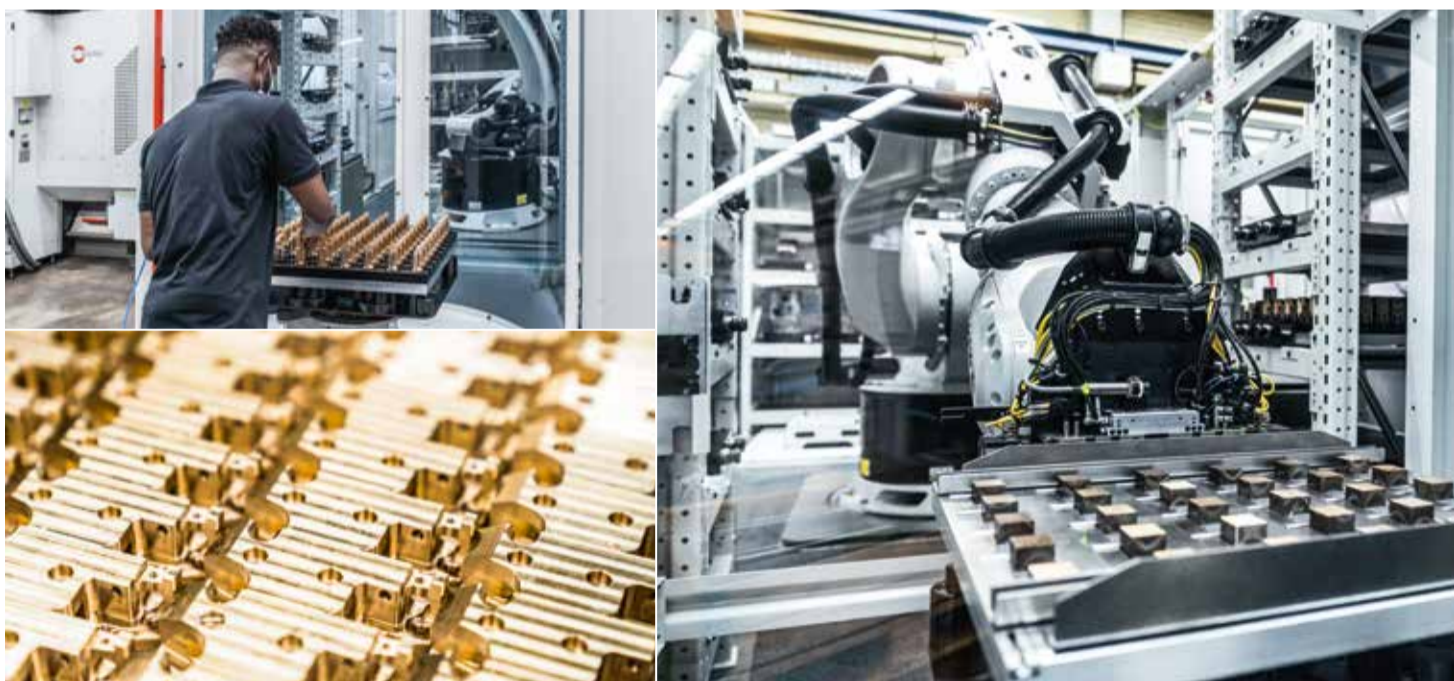
top Operator Samuel Emeka checks a die with finished components for Hohner's narrow stitching heads. right The new Hermle system replaces six individual machines and is significantly more productive thanks to robot automation. bottom In addition to cast iron, plastic, aluminium and steels, Hohner Maschinenbau also machines brass on the C 400 U and C 650 U.
