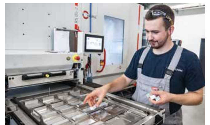
top Fadri Pitsch loads the dies with blanks, thereby providing the C 12 U with enough work for the next unmanned shift.
