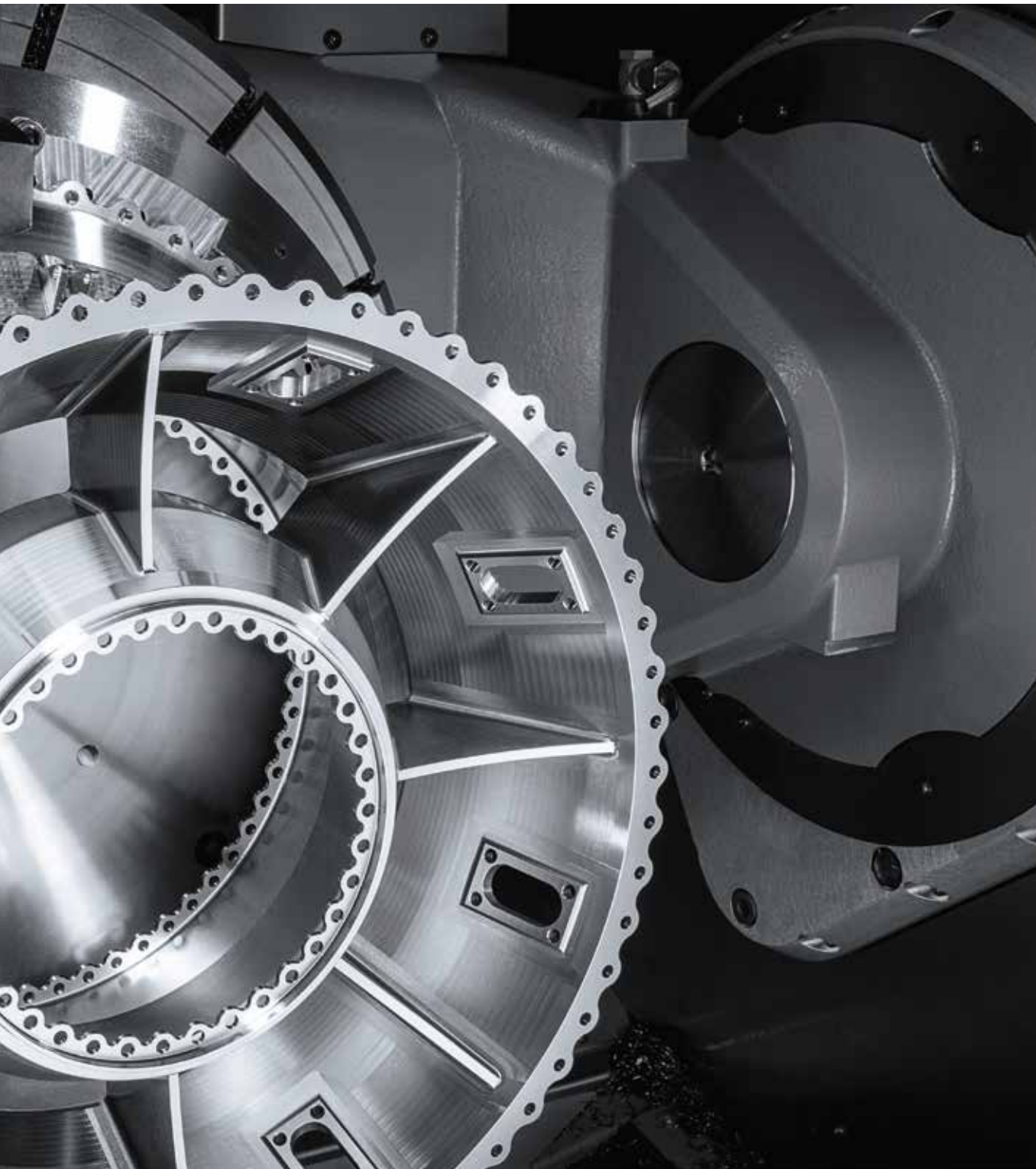
Hermle C 42 U MT dynamic in 5-axis mill/turn version | Machining of a engine casing for the aerospace industry.
